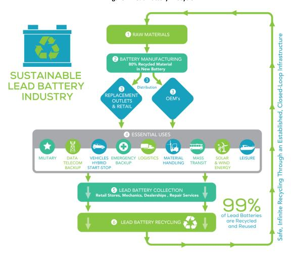
Figure 1. Lead Battery Lifecycle
